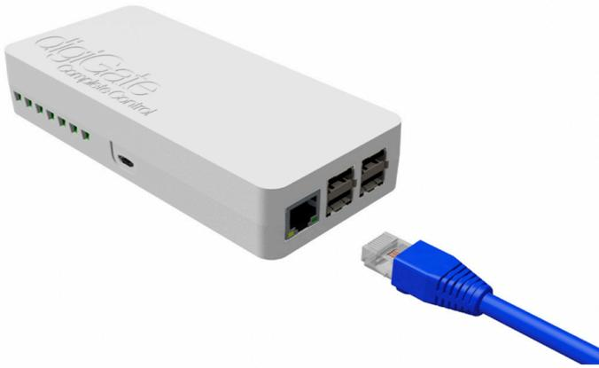
**Step 2:** Plug the other end of the cable into your router, access point, network switch or ethernet-over-power (powerline) device.
